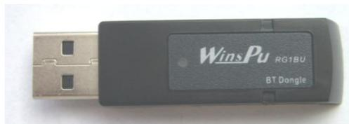
Insert the BT dongle into the USB port of PC. The lower right corner of screen will show the icon
